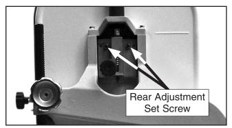
Figure 71. Rear lateral adjustment set screw.
